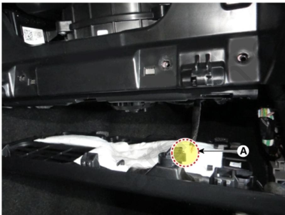
8. Separate the glove box housing (A) after loosening the mounting screws, bolts, and nuts.
