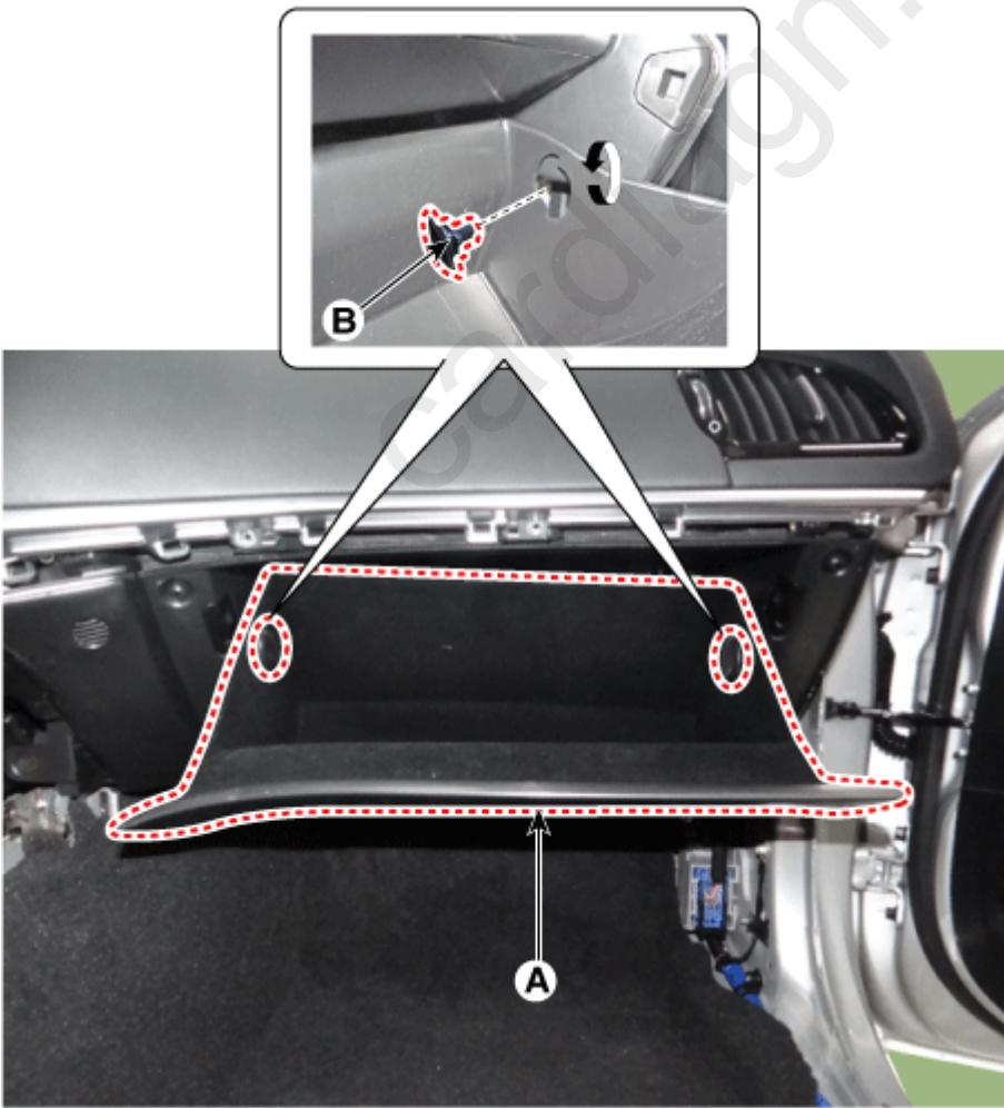
4. Remove the air damper (A) from the glove box (B).
