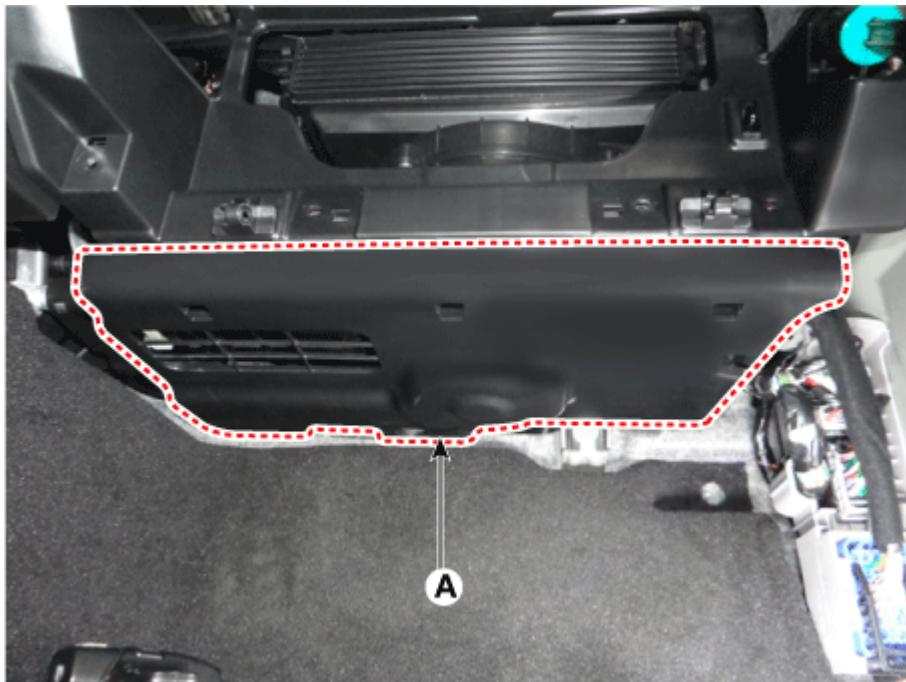
7. Disconnect the lamp connector (A) and remove crash pad under cover.
