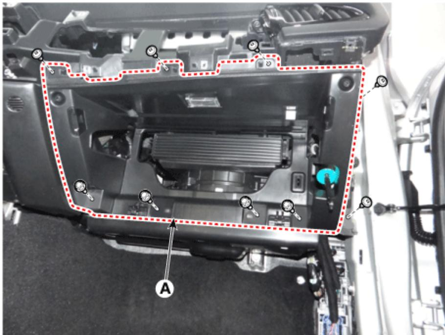
9. Remove the glove box housing after disconnecting the connector (A), (B).
